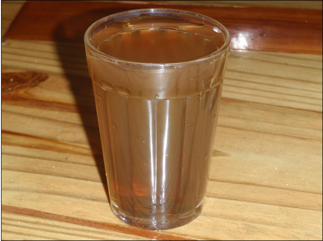
Figure 4b. After addition of bleach, the same reddish-brown color (see Fig. 4a) is visible in water from a dug well in the village of Santa Rita, downstream from the Santo Antônio tailings disposal facility at the Kinross Gold Morro do Ouro mine in Paracatu, Minas Gerais, Brazil. The bleach re-oxidizes the dissolved metals to form fine-grained particles of metal oxides and oxyhydroxides. Photo taken by the author on May 6, 2019.
