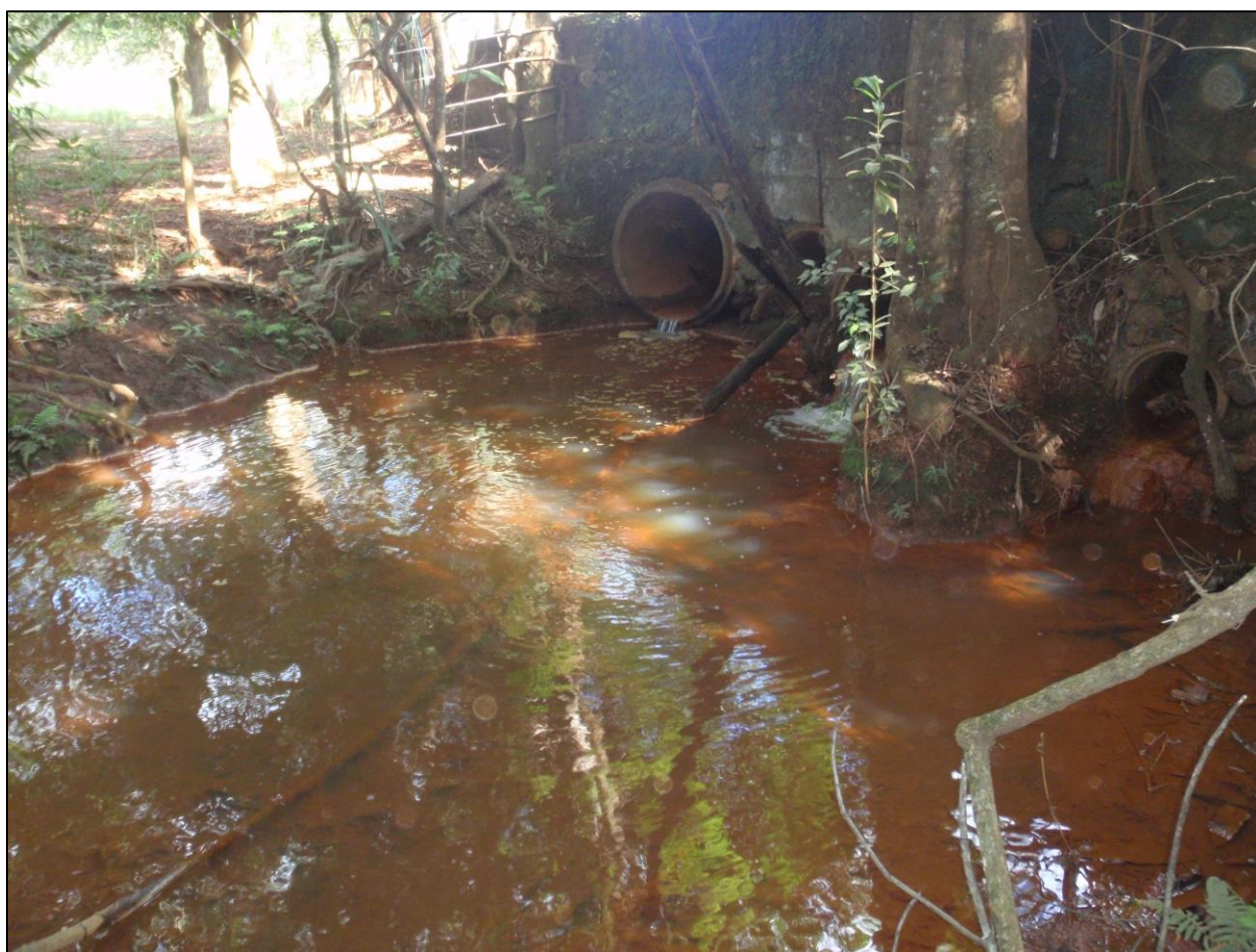
Figure 4a. Acid mine drainage is evident in the reddish-brown color in the discharge from the Santo Antônio tailings disposal facility at the Kinross Gold Morro do Ouro mine in Paracatu, Minas Gerais, Brazil, even after water treatment to remove the acidity. The pipe in the background is a culvert under the highway. The stream on the other side of the highway receives the discharge from the tailings disposal facility. The reddish-brown color results from fine-grained particles of metal oxides and oxyhydroxides. Photo taken by the author on May 7, 2019.
